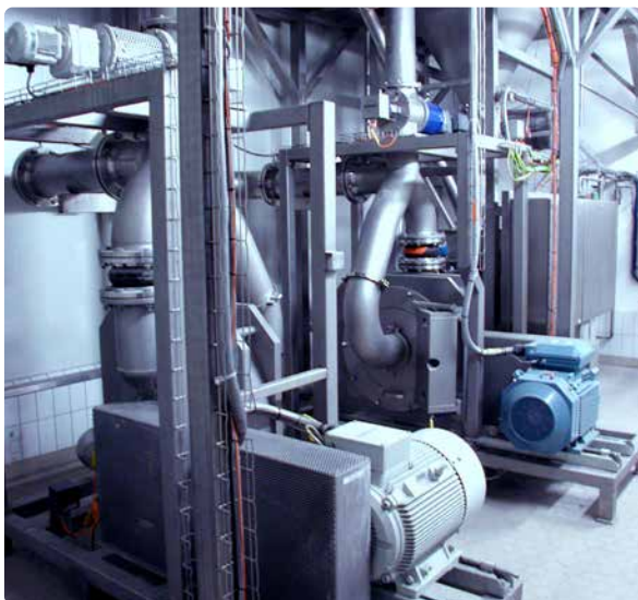
REKORD 630 GMP fine grinding system for lactose
